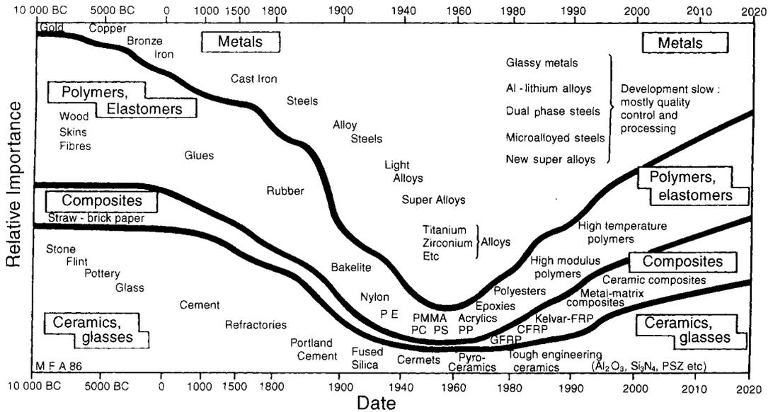
**Fig. 1.2** The evolution of engineering materials with time. 'Relative Importance' in the stone and bronze ages is based on assessments of archaeologists; that in 1960 is based on allocated teaching hours in UK and US universities; that in 2020 on predictions of material usage in automobiles by manufacturers. The time scale is non-linear. The rate of change is far faster today than at any previous time in history.
